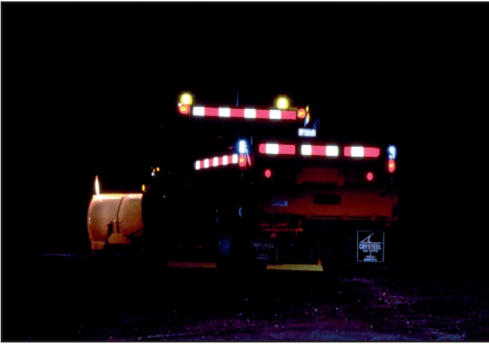
Studies show that heavy trucks with reflective markings experience 20% fewer nighttime collisions.
