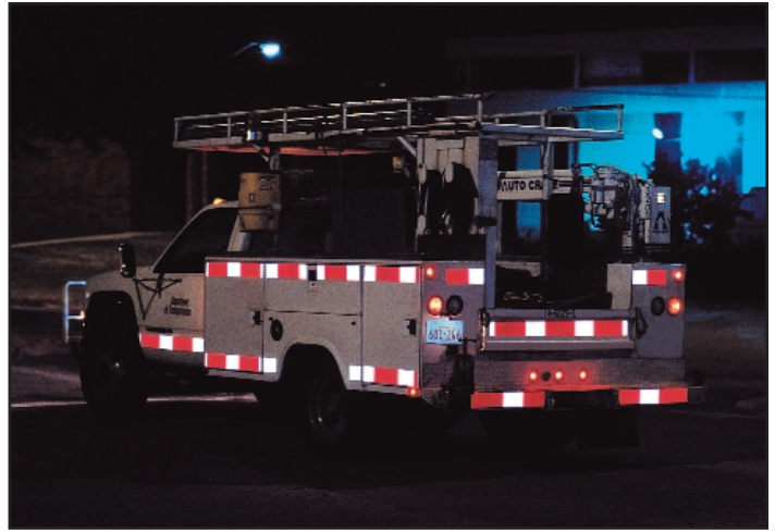
Marked vehicles are clearly visible even when backing up, crossing traffic or making turns.
