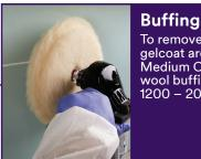
To remove sand scratches, buff the sanded gelcoat area with 3M<sup>™</sup> Perfect-It<sup>™</sup> Gelcoat Medium Cutting Compound + Wax and a white wool buffing pad. Set the buffer speed between 1200 – 2000 Max. RPM.
