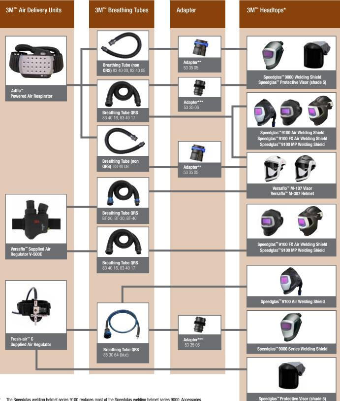
\* The Speedglas welding helmet series 9100 replaces most of the Speedglas welding helmet series 9000. Accessories and spare parts for the 9000 helmets will be available for 3-5 years.
